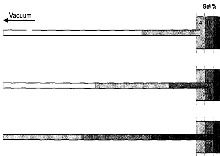
Fig. 1. Illustration of the micro-reservoir system used to cast step gradients in the capillary. Each reservoir chamber was separated by parafilm and filled with gelling solutions containing the different monomer concentrations. To change the composition of the solution drawn into the capillary, the parafilm was pierced and the capillary inserted into the next chamber.
